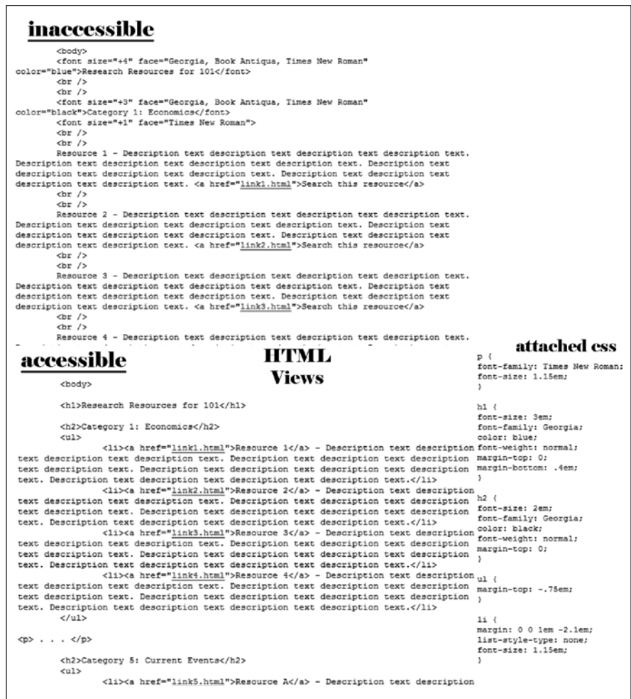
Figure 2. Here we see distinct variances in the source code. The image at the top (inaccessible) reveals code that does not use headings or unordered lists for each resource. The image on the bottom (accessible) does use semantically correct code, maintaining the same look and feel of the headings and list items through an attached cascading stylesheet.
